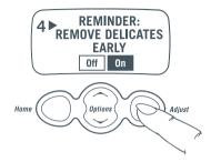
To activate the reminder, scroll to Options screen 4, press the ADJUST button to select **ON**, then press **HOME** to save your setting.
